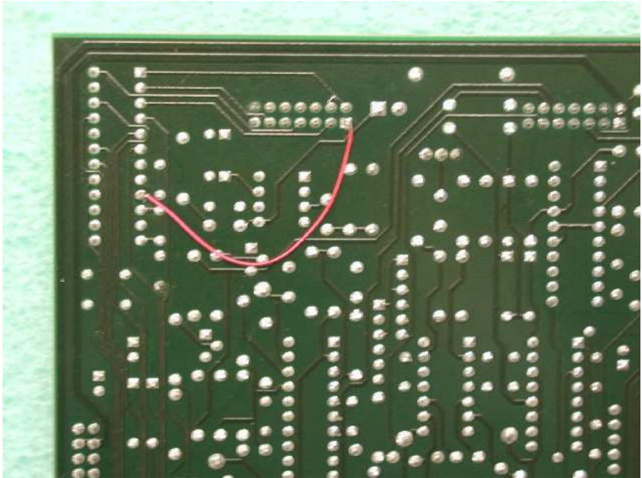
On the connector board, connect the "EXT SPKR" signal to pin 1 on J2. This connection can be made on the back side of the board. Also connect VCC from pin 1 on JS1 to pin 4 on J2. This connection requires routing the wire through one of the unused holes in J12 between front and back sides. The following pictures show these connection on the DDF6114D board.
