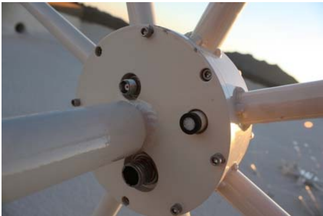
Figure 4: Secure the lower mast to the frame using the cap screws
