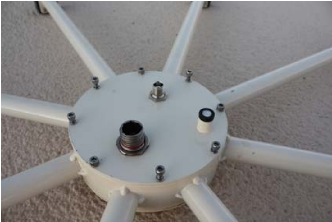
Figure 3: Remove the longer cap screws to install the lower mast
