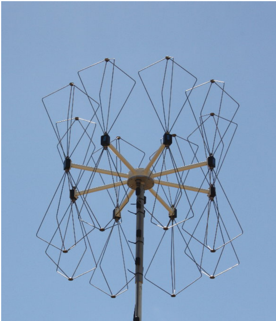
Figure 9: Fully Assembled VHF Antenna
