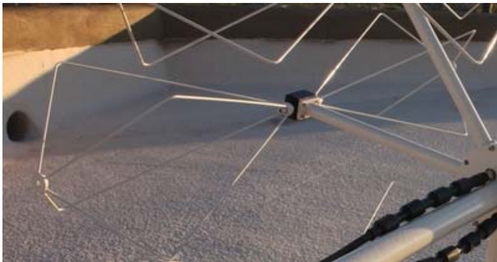
Figure 8: Antenna element mounted on the balun
