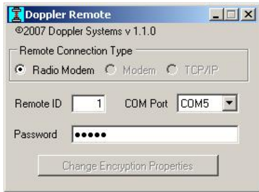
Figure 19: Set the Remote ID to a Number Unique From All Other Mobiles on the Network
