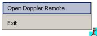
Figure 18: Right Click the Doppler Remote Tray Icon to View Doppler Remote Dialog
