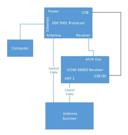
Figure 1: Wiring Diagram for Doppler Direction Finder with ICOM R8600 Receiver
