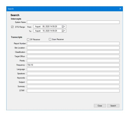
To extract the data for a given time period click on the DTG Range and enter the desired date/time range. To extract data recorded on a given frequency in a certain time period then enter the frequency as well. Press Search to display a dialog similar to the one below and click the Check All button.
