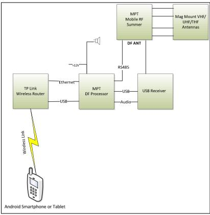
Figure 1: Block Diagram of Hardware Setup
