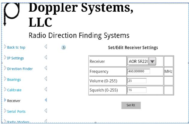
Figure 6: Setting the Receiver Using a Web Browser
