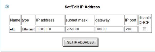
**Figure 4: Default IP Parameters**
